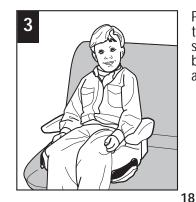
Place child restraint against the back of the vehicle seat. Place the child's bottom and back flat against the child restraint.
